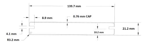
Figure 4. "DecKorators® Vault," "DecKorators® Voyage" and "DecKorators® Frontier" grooved profile
