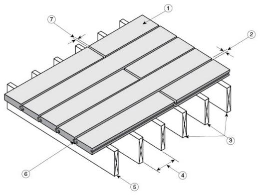
Figure 1. "DecKorators® Vault," "DecKorators® Voyage," "DecKorators® Frontier," "SLS" and "Ultra Light" composite deck boards with hidden fastener system
