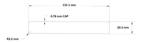
Figure 5. "SLS" and "Ultra Light" solid profile
