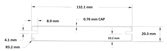
Figure 6. "SLS" and "Ultra Light" grooved profile
