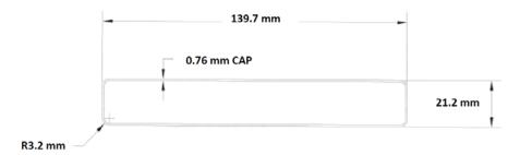
Figure 3. "DecKorators® Vault," "DecKorators® Voyage" and "DecKorators® Frontier" solid profile
