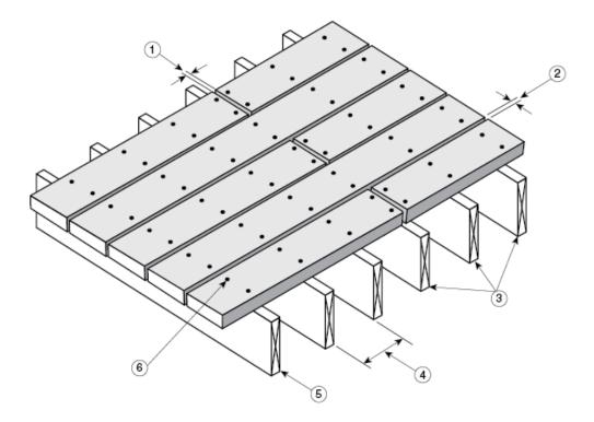
Figure 2. "DecKorators® Vault," "DecKorators® Voyage," "DecKorators® Frontier," "SLS" and "Ultra Light" composite deck boards with fasteners
